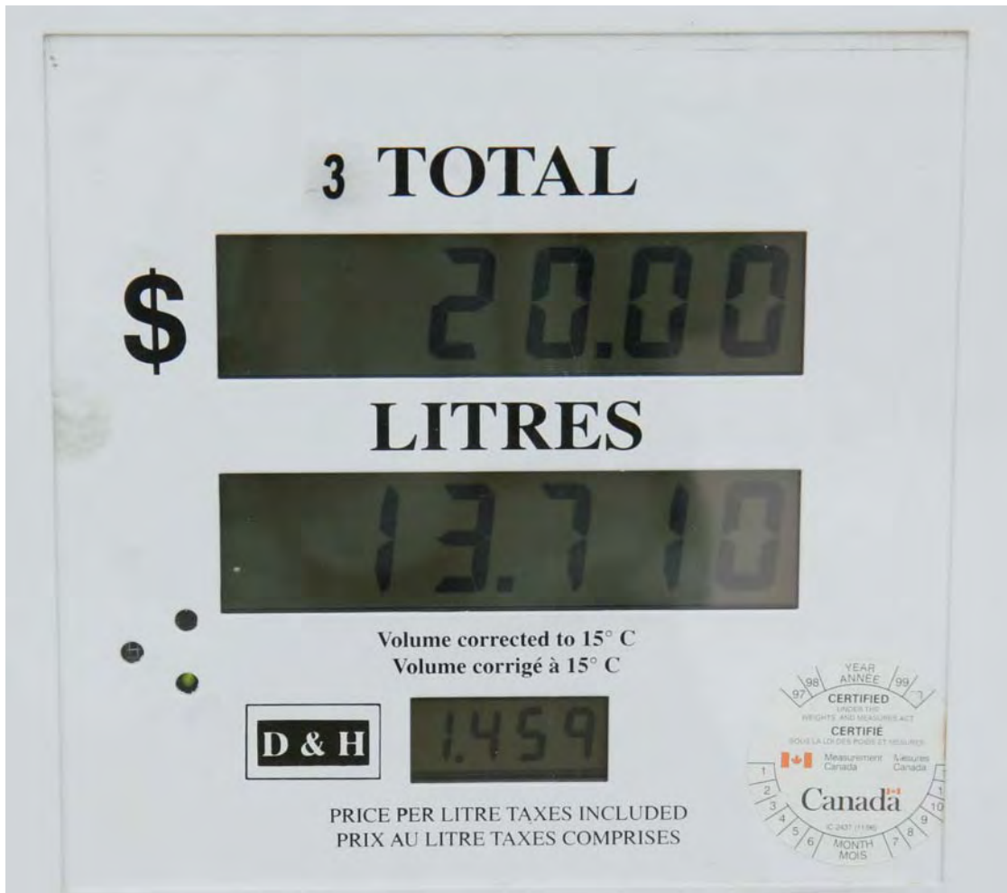
Fuel dispenser in Waterton, Alberta (Canada) displays temperature correction labeling in French and English. Photo Credit: Gordon Schremp, California Energy Commission.
